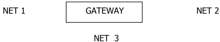
Gateways connect two networks that are heterogeneous in nature. (That is a network differing in IP).
